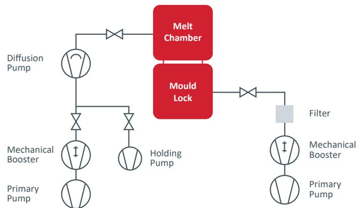
Typical layout for PIC operation
